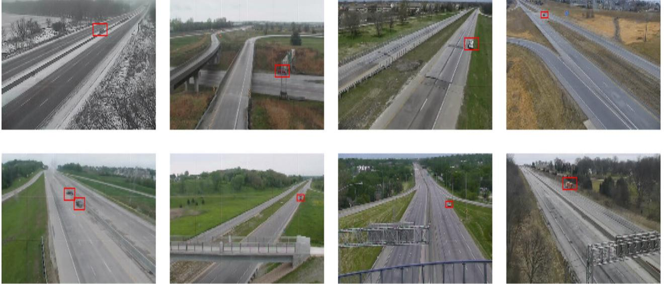
Figure 6. Sample correct results (true positives) achieved by our method. The red boxes represent the anomaly detected when a vehicle is stopped on the road.
